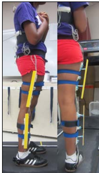
Figure 4.4 Bright color extensions (off-set by 5 cm) were attached to orthoplast sticks that hold infrared markers on legs and tights.
